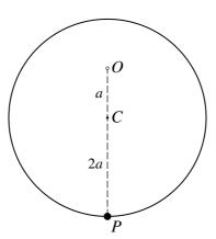
A uniform solid sphere with centre C, radius 2a and mass 3M, is pivoted about a smooth horizontal axis and hangs at rest. The point O on the axis is vertically above C and OC = a. A particle P of mass M is attached to the sphere at its lowest point (see diagram). Show that the moment of inertia of the system about the axis through O is  $\frac{84}{5}Ma^2$ .
